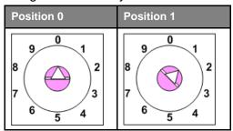
**NOTE**: To avoid damaging the rotary switch, use a screwdriver to change the position.
