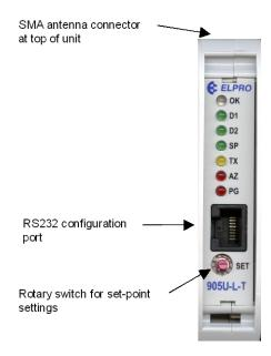
The triangle on the rotary switch indicates the current position, for example:
